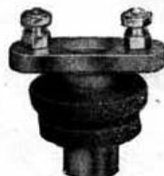
EDDYSTONE All-Wave H.F. Choke. Low loss D.L.-9 former with two section honeycomb wound coils. One screw fixing. Waverange 12.5 to 2,000 metres. Self capacity 2.4 m.mfd. Inductance 17.9 millihenries. D.C. resistance 60 ohms. No. 1066 ... 2/3
