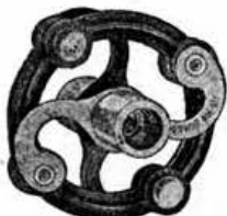
EDDYSTONE Flexible Coupler. Free from backlash but very flexible, this coupler banishes alignment troubles. D.L.-9. H.F. Insulation. For 1-in. spindles. No. 1009 ... 1/8
